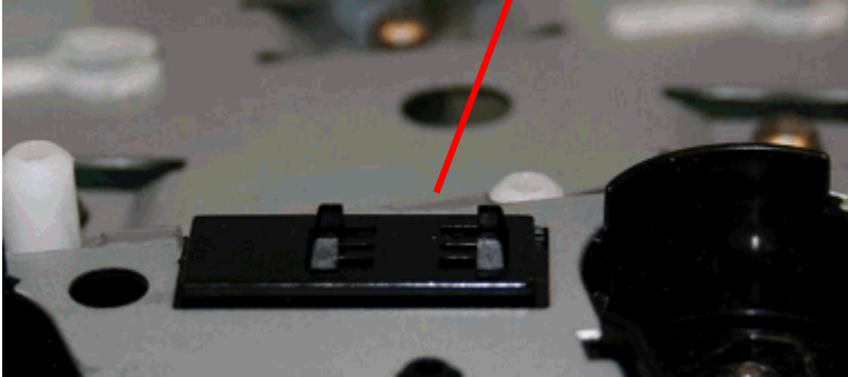
Figure 4: Troubleshooting cartridge / drum sensor
