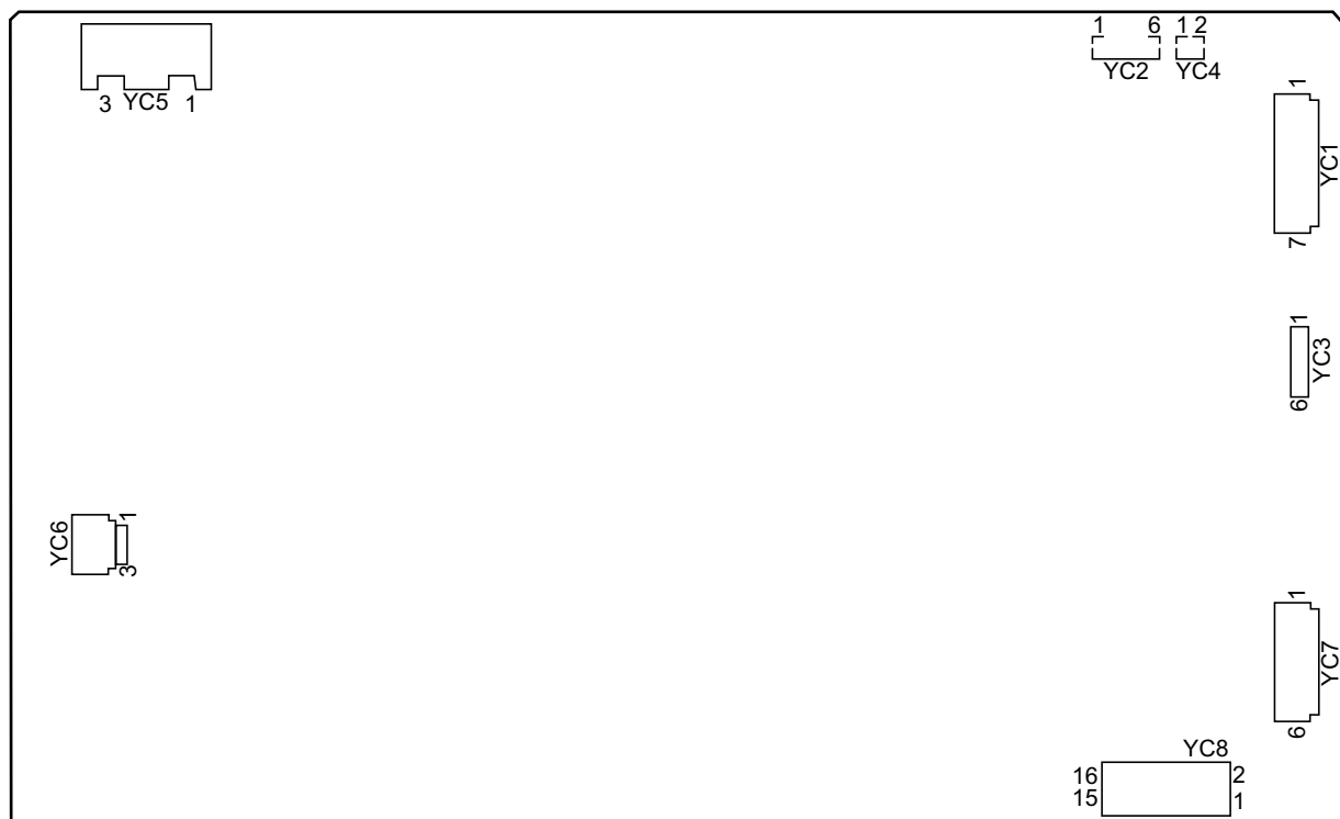
Figure 2-3-2 Power source PWB silk-screen diagram
